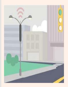
Small cells are just like the name implies – short range cell sites used to complement macro cell towers in a smaller geographic area ranging from a few hundred feet to upwards of 1,000 feet. These lower power antennas enhance capacity in high traffic areas, dense urban areas, suburban neighborhoods, and more. Small cells use small radios and a single antenna placed on existing structures including utility poles and street lights.
